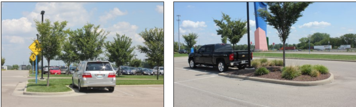
Figure 1115-B: Landscaping and screening is intended to soften the appearance of large expanses of parking areas and can also provide areas for stormwater management.
