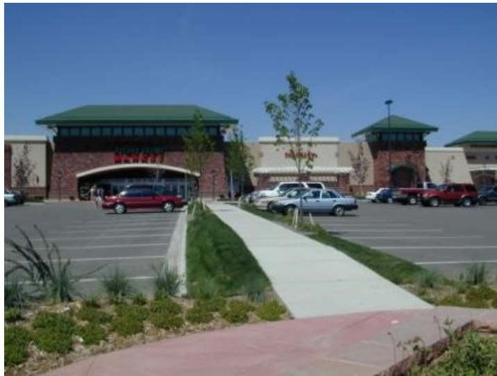
Figure 1117-E: This photograph illustrates how a sidewalk connecting the public sidewalk to the business can be integrated into the required landscaping.
