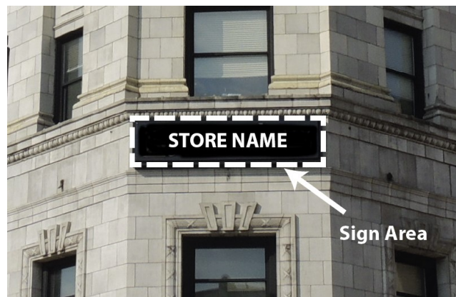
Figure 1119-C: Illustration of computing the sign area for wall signs with a background panel or cabinet.
